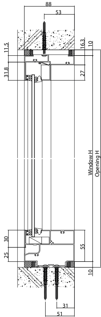
Vertical section: Single fixed window
